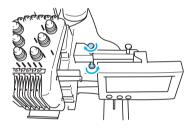
Adjust the orientation of the operation panel. Loosen the thumb screw, adjust the operation panel to an easy-to-view orientation, and then tighten the thumb screw.
